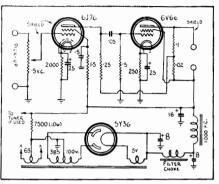
Here is the circuit of the amplifier. If a radio tuner is used, the 7500 ohms resistor may be omitted, and the tuner adjusted so that its average drain is equal to 35 mills. This will ensure the voltages being correct, and also provide sufficient energisation for the field. Although the 7500 resistor is shown as 10 watt, a 20 walt type will keep cooler and costs little more.
